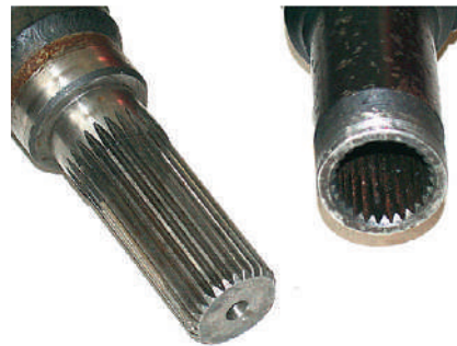
Figure 5.89 A splined joint connects to the gearbox
